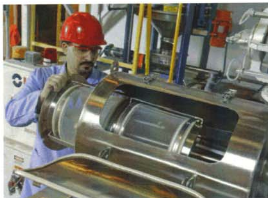
Cylindrical screen and helical paddles slide out of the Centri-Sifter MO screener end for thorough washdown and rapid screen changes.
