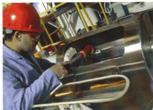
Screening chamber door of the Centri-Sifter MO screener provides quick access for cleaning, inspection.
