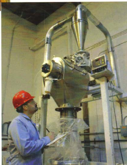
On-size particles are gravity discharged through the main outlet, while agglomerates propelled through the end of the cylindrical screen are discharged through a smaller end spout.
