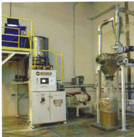
Polisher (center) is a continuous inline mixer that improves the flow properties of materials. After mixing and surface-smoothing, particles are transferred to a Centri-Sifter MO screener (right) for scalping of agglomerates.
