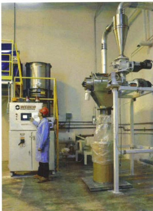
The 'Polisher' feeds material in-line to Centri-Sifter MO centrifugal screener that separates on-size particles from oversize agglomerates.
